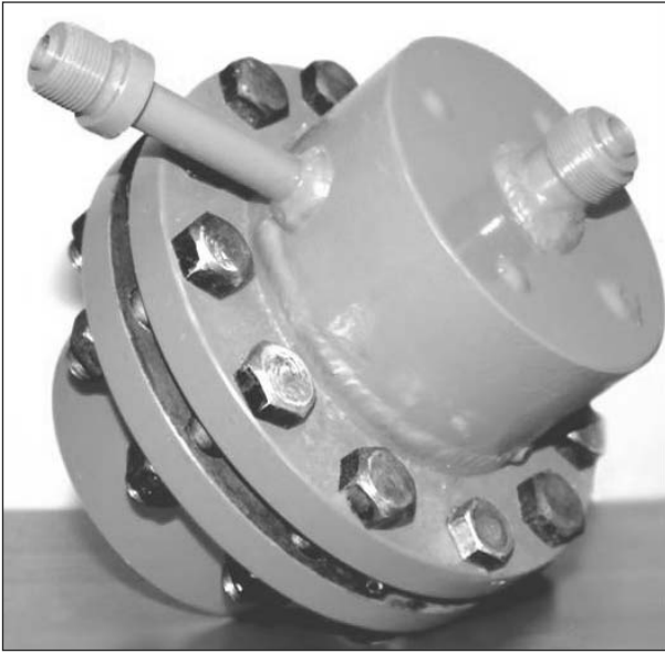
Fig. 2. Photo of the exploratory prototype of turboimpact oil separator of compressed gases of breathing system of GTI of closed cycle
