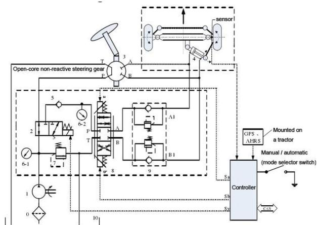
**Fig. 1.** Diagram of the hydraulic steering system with intelligent control of agricultural machinery
