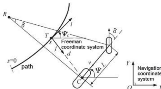
Fig. 3. Relative movement and position relationship between agricultural machinery and path
