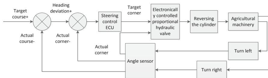
Fig. 2. Steering PID control principle
