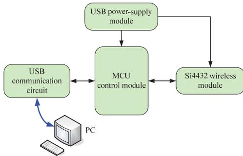
Fig. 4. Hardware of terminal node
