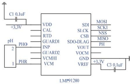
Fig. 3. pH acquisition circuit
