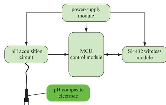
Fig. 2. Hardware of acquisition node
