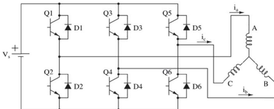
Fig. 2. Simplified BLDC drive scheme
