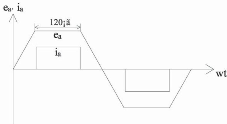
Fig. 1. One phase square wave current and trapezoidal wave back electromotive force waveform
