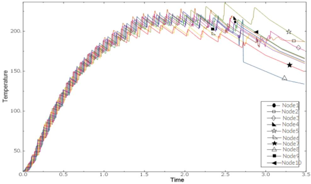
Fig. 6. Temperature of circumferential nodes in the same radius on the surface of the brake disc
