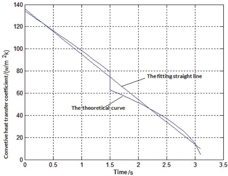
Fig. 4. Convective heat transfer coefficient with braking time of the brake disc's radiating surface
