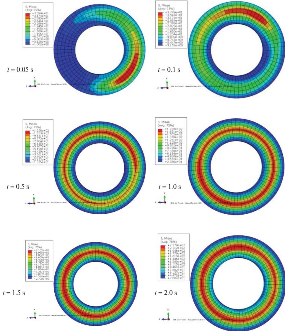
Fig. 7. Stress field distribution of the brake disc at different moments time
