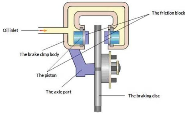
Fig. 1. Structure of disc brake
