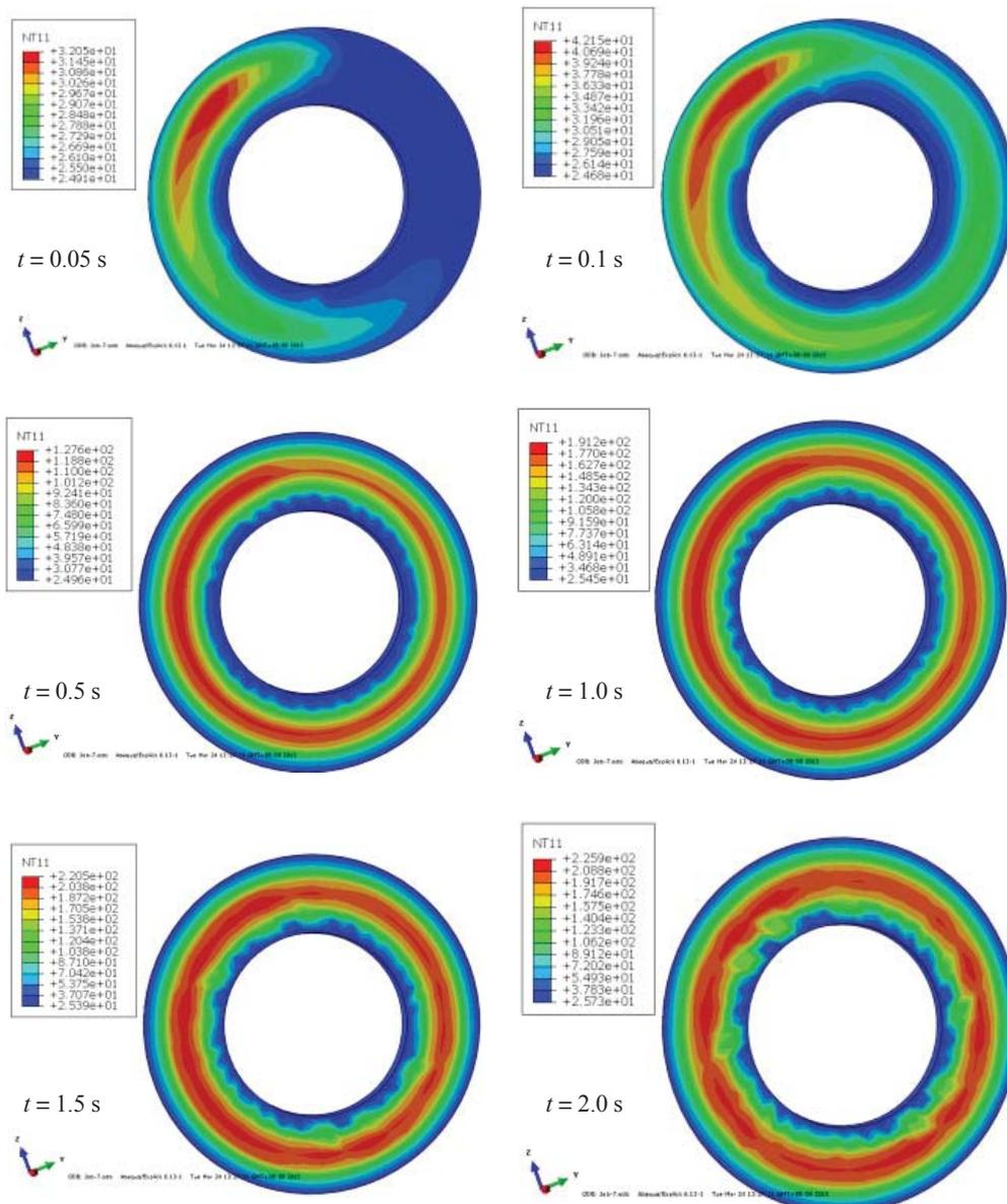
Fig. 5. Temperature field distribution of the brake disc at different moments of time
