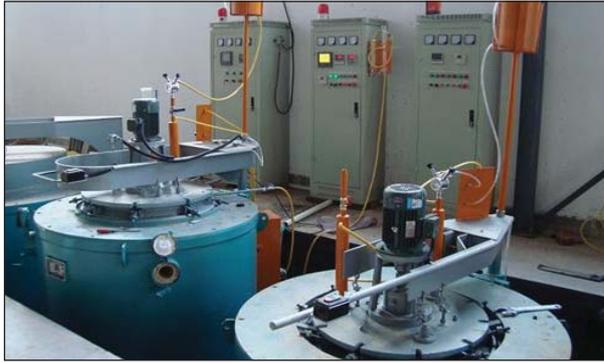
Fig. 4. Computer-controlled crankshaft gas soft nitriding
