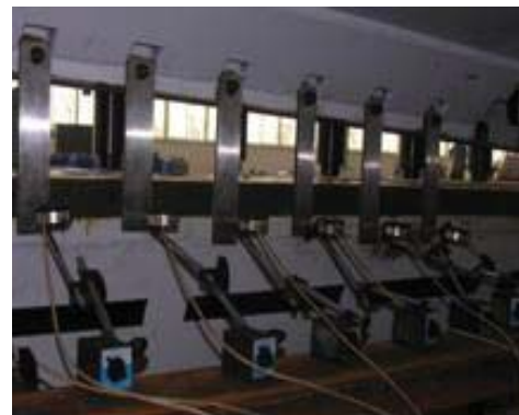
Fig. 2. Meters installed on the upper blade
