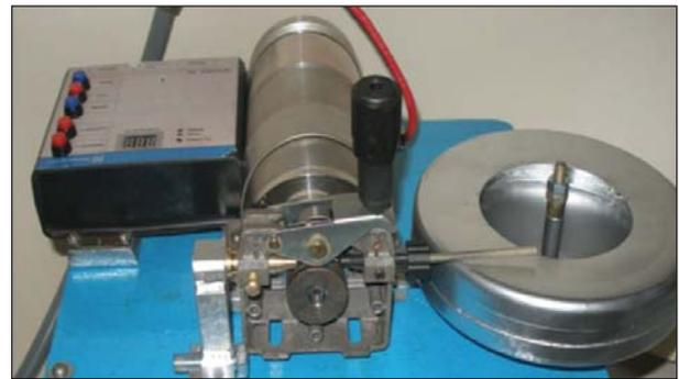
**Fig. 1.** Layout of the MPWF based on of the valve electric drive “Impuls-2 PM-80”
