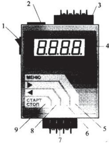
**Fig. 3.** Appearance of the electricity consumption meter with indication of controls and terminals
