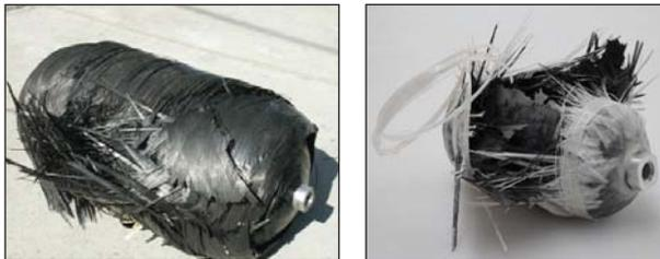
Fig. 6. Results of kevlar composite tank explosion
