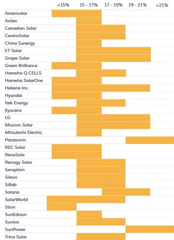
Fig. 2. Solar photovoltaic panels efficiency
