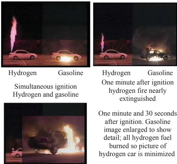
Fig. 5. Illustration of gaseous hydrogen ignition and burning compare with gasoline
