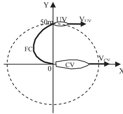
**Fig. 8.** Scheme of the UV movement around the CV along a circle
