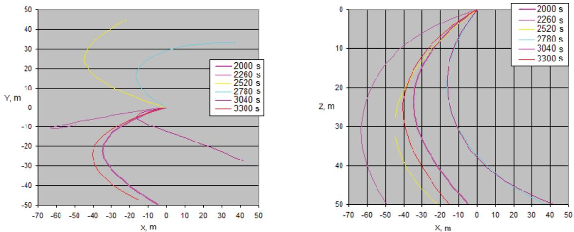
**Fig. 13.** Change in the shape of the FC connecting the CV and the UV during the UV movement projected onto the  $XOY$  and  $XOZ$  planes (modeling results for Option 4)
