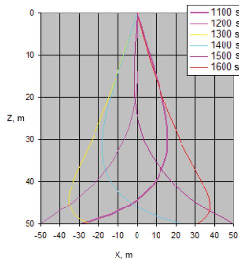
**Fig. 6.** Change in the shape of the FC connecting the CV and the UV during the UV movement projected onto the  $XOY$  and  $XOZ$  planes
