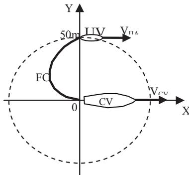
**Fig. 5.** Scheme of the UV movement around the CV along a circle
