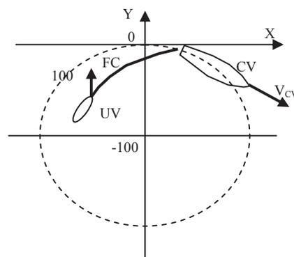
**Fig. 20.** CV moves along a circle with the radius of 100 m at the speed of 1 m/s, and the non-self-propelled UV moves behind it tied to a FC 100 m long
