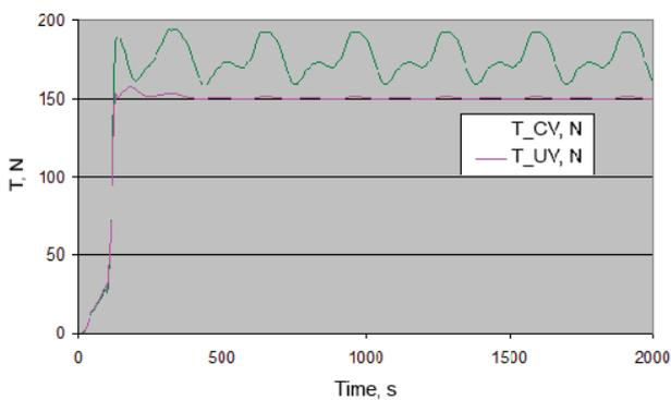
**Fig. 19.** Forces of tension acting on the CV and the UV
