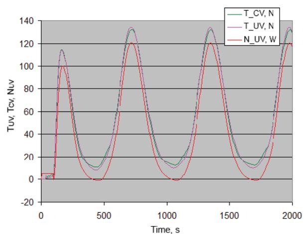
**Fig. 10.** Change in the force of the FC tension acting on the CV and the UV
