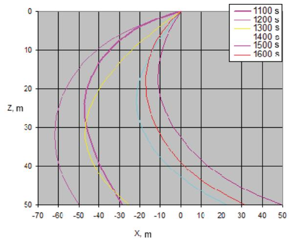
**Fig. 9.** Change in the shape of the FC connecting the CV and the UV during the UV movement projected onto the  $XOY$  and  $XOZ$  planes
