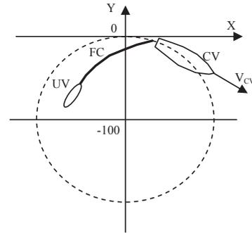
**Fig. 17.** CV moves along a circle with the radius of 100 m at the speed of 1 m/s, and a non-self-propelled UV moves behind it tethered by a FC 100 m long
