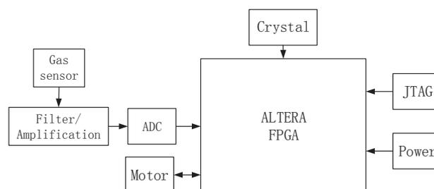
Fig. 2. Hardware component of the system
