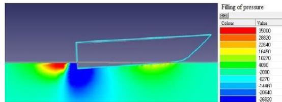
Fig. 6. Pressure distribution along the planning vessel surface
