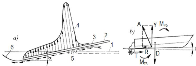
**Fig. 1.** Scheme of the hydrodynamic pressure effect on the planning plate (a) and the force on the bottom of the planning cutter (b) [1].
